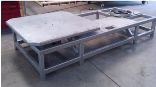
Stainless Steel dual deck power turntable for 3500 lbs pallet conveyor system
