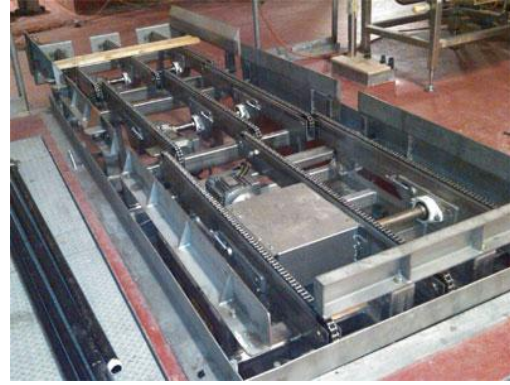
Stainless Steel multi strands chain conveyor for 3500 lbs pallets
