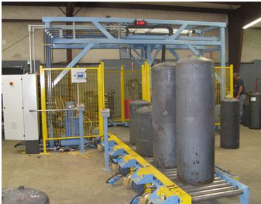
Tanks automatic downending conveyor system
