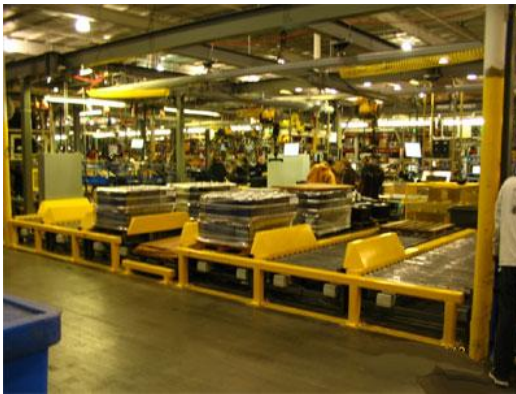
Pallets zoned conveyor system
