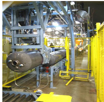
Tanks automatic downending system
