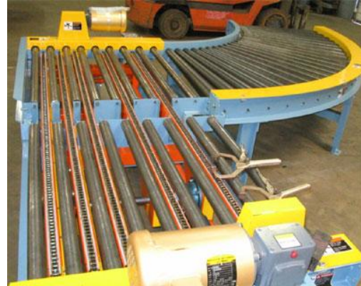
Crossover conveyor system
